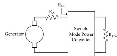
Fig. 5: Using a power converter to get optimal power transfer from the generator
