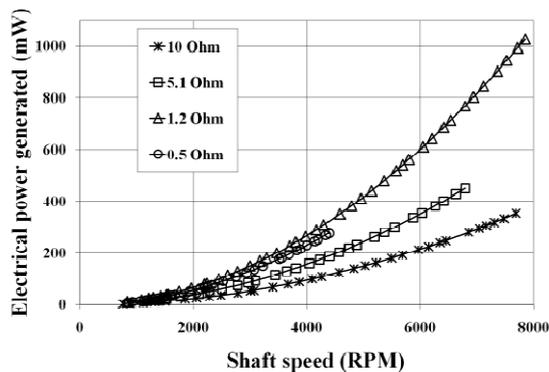
Fig. 3: Measured powers for the specified load resistances when  $R_A = 1.1 \Omega$
