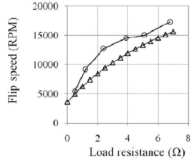
Fig. 4: Flip-over speed vs. load resistances when  $R_A = 1.1 \Omega$ : experimental (circles) and modelled (triangles)
