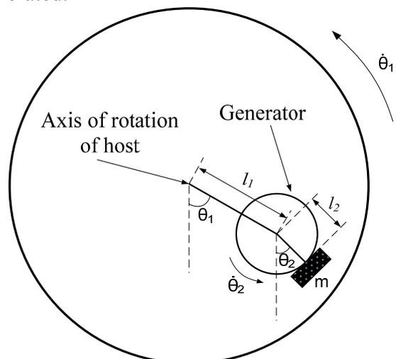
Fig. 8: Schematic of the off-axis generator
